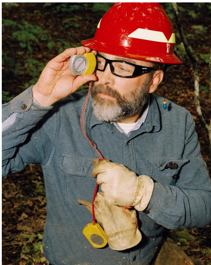
Michael Stambaugh looks through a clinometer, an eyepiece that uses triangulation to measure tree heights, vertical angles, and slope steepness.
